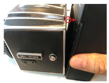
I. Align the camera body latch with the small hole on the Hasselback, keeping the angle parallel.
